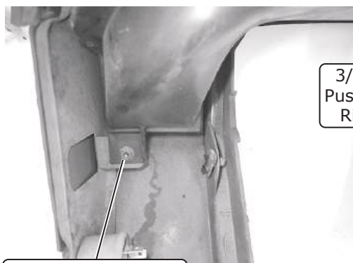
Remove mounting hardware to remove OEM plenums
