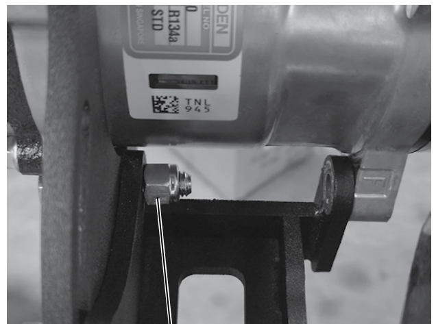
Secure bolt with 3/8-16 locknut. Leave loose.
