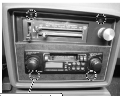
Remove control panel/radio bezel by removing (4) screws
