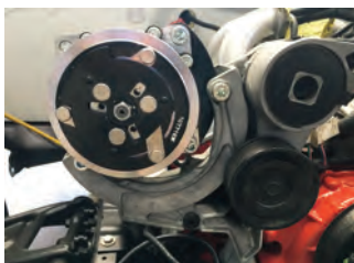
141805 Sanden type / R4 multi-groove conversion bracket. (1988-95 Chevy truck small block with stock height valve covers).
