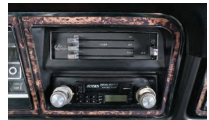
1973-86 factory-look replacement control panel installed
