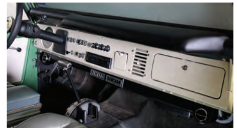
Ford Bronco dash with SureFit system full width plenum, controls and Vintage Air louvers, (4-vent kit also available)
