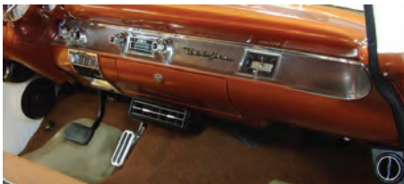
1957 Chevy installation with center plenum
