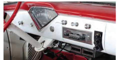
1955-59 Chevy Truck dash with SureFit kit and standard rotary replacement control panel
