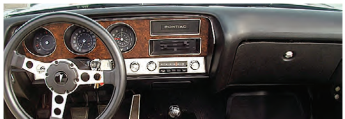
1972 GTO factory air dash shows Vintage Air OEM look controls and the system uses the factory air conditioning vents.
