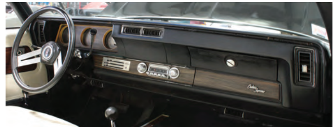
Cutlass factory-air dash with Vintage Air OEM look control panel. SureFit installations in factory-air equipped cars use the original in-dash A/C louvers)
