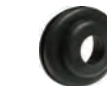
33137-VUI Rubber grommet inner hole size .625" (will expand to 1"), 1.75" O.D. - drill hole size 1.25"
