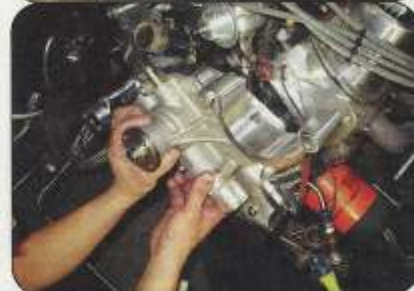
More black RTV is applied to the mounting surfaces of the new timing cover and the water pump. The gasket is applied, and the water pump is bolted into place.
