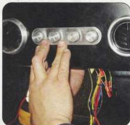
After everything checked out, Mosco unplugged the wiring, installed the controls in the dash, and then plugged in all of the wiring again.
