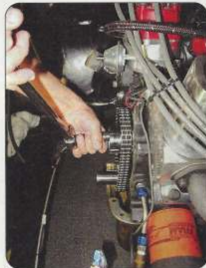
While the center console was being removed, the accessory system, timing cover and fuel pump drive were being removed from the Ford engine.
