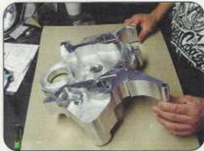
The next order of business was to prep the new Vintage Air timing cover that has all the mounts for the alternator, air conditioning compressor, power steering pump and water pump built right in.
