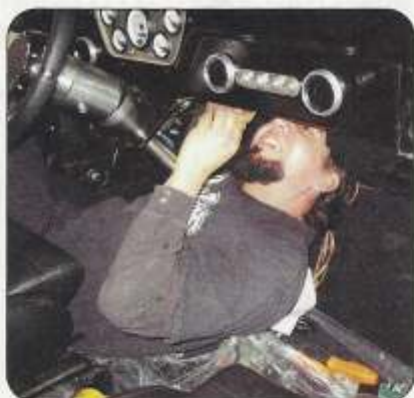
After everything checked out, Mosco unplugged the wiring, installed the controls in the dash, and then plugged in all of the wiring again.
