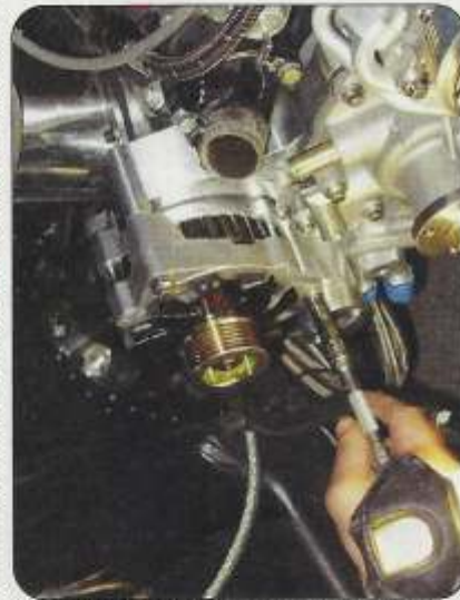
The new alternator is mounted to the Vintage Air timing cover/engine accessory mount.
