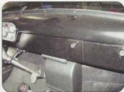
Because the center of the dash had already been shaved, they decided that the vents and controls for the Vintage Air setup would fit great in the center of the dash.
