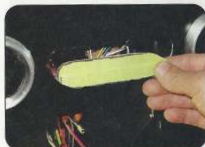
The section that had to be cut out for the controls was cut with a body saw, and a hand file was used to clean up the edges.
