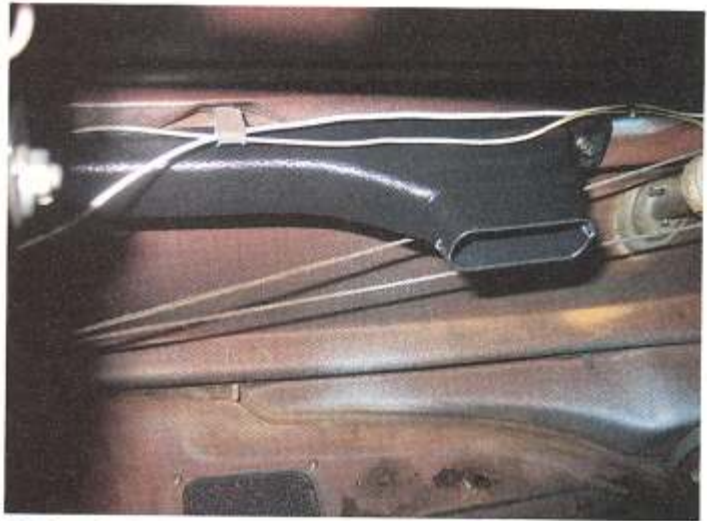
Moving under the dash, you'll attach the defroster duct in the correct location.
