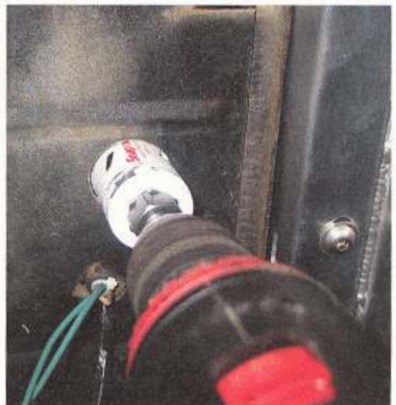
It will be necessary for you to drill a hole through the core support for the A/C lines.
