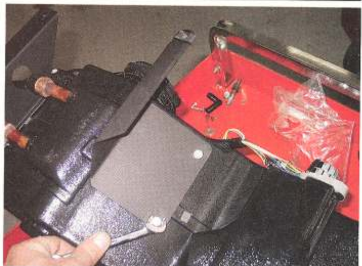
Next you'll bolt up the evaporator bracket to the evaporator itself. This will allow you to secure it tightly under the dash.
