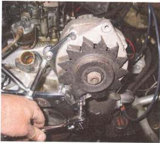
The alternator bolts up to the other end of the bracket using more of the Vintage Air-supplied hardware.
