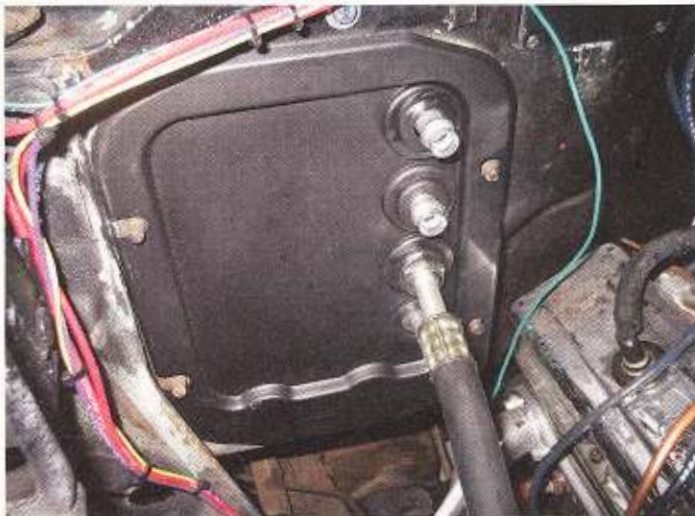
Then attach the new firewall block-off plate to the firewall. The two upper ends are where you'll attach the heater hoses and heater-control valve.
