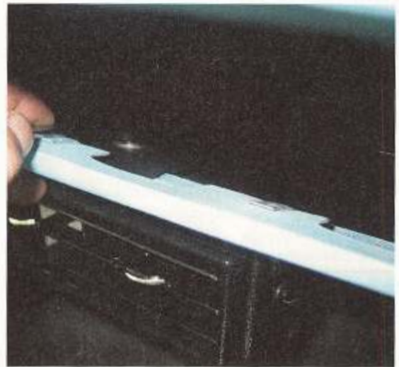
With the glove box removed, you'll mount the center register duct to the bottom of the dash.
