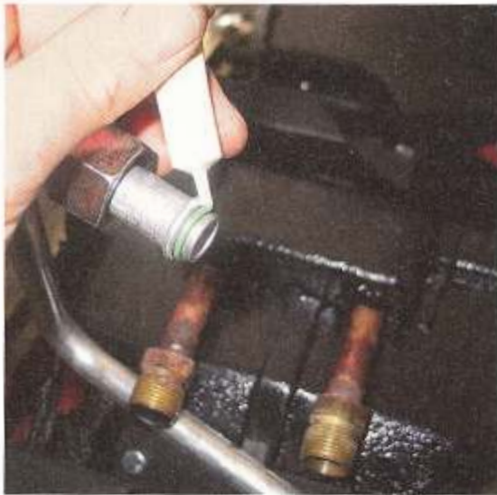
Be sure to use the tube oil that is supplied on all of the O-rings in the new system.
