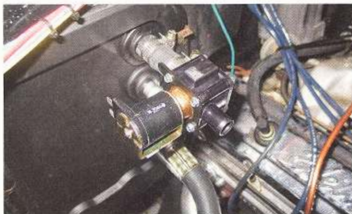
Here's how the heater-control valve looks all bolted up.
